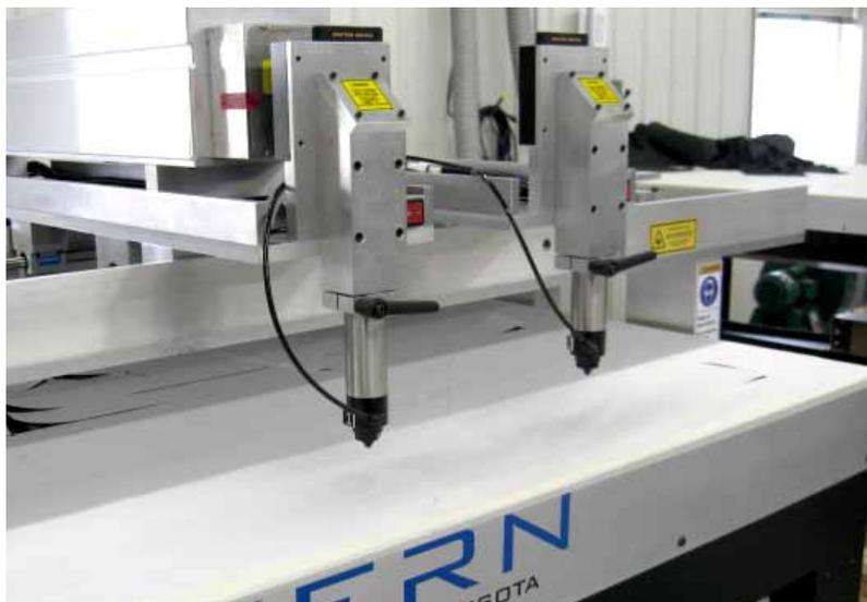
All Kern Standard Laser Systems can be equipped with dual laser heads to double your production. KCAM laser software will control each laser separately so both can be tuned to equal power. The slave laser connects to the master laser via an adjustable bar. The bar can be removed and the slave laser can be locked to the far right of the gantry allowing the master laser with full use of the laser table.
